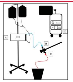
Illustration showing the automated pressure control system. Color coding in this illustration is not intended to be universal with systems in existence. Blue line indicates flow into the joint, and red lines indicate flow out of the joint. **A**, Automated pressure control pump, (**B**) pressurized inflow, (**C**) a source of outflow, and (**D**) arthroscopy console tower for light source and motorized equipment (eg, shaver).
